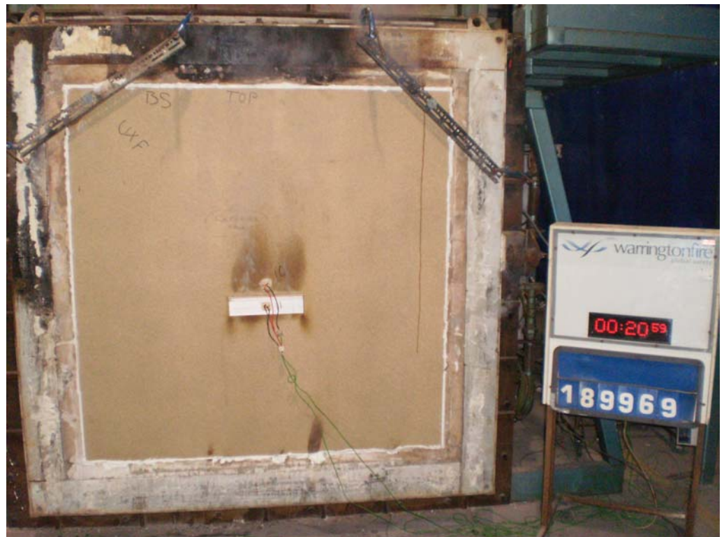
The unexposed face of the assembly after a test duration of 20 minutes
