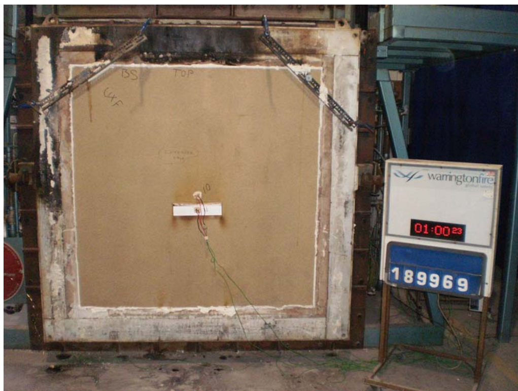
The unexposed face of the assembly after a test duration of 60 minutes
