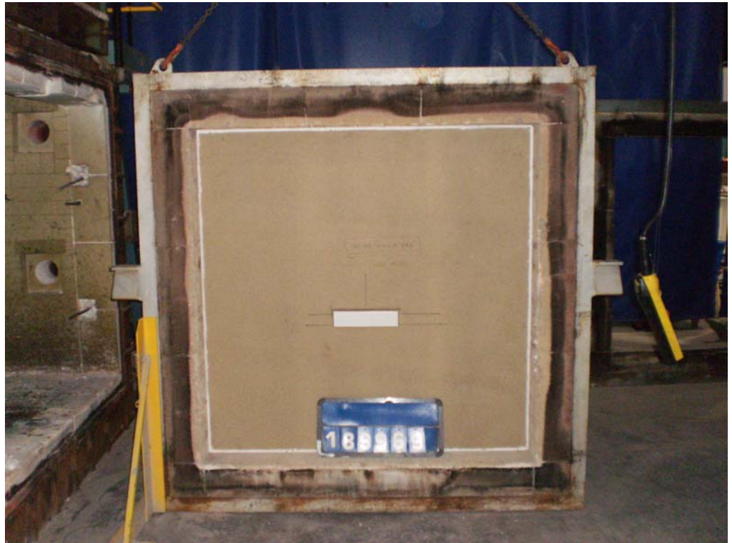
The exposed face of the assembly prior to the start of the test
