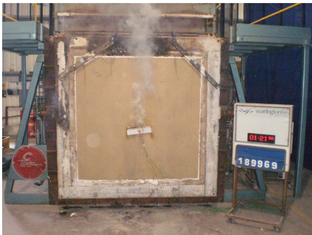
The unexposed face of the assembly after a test duration of 81 minutes
