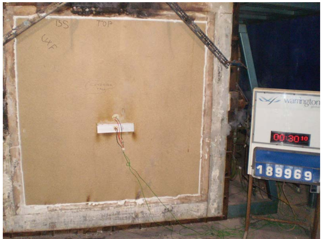
The unexposed face of the assembly after a test duration of 30 minutes
