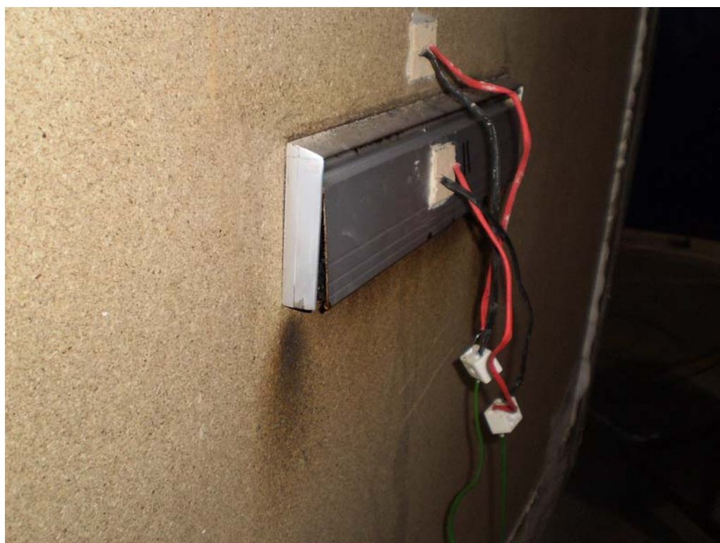
The bottom edge of the letterplate flap starts to get pushed open with the reaction of the intumescent
