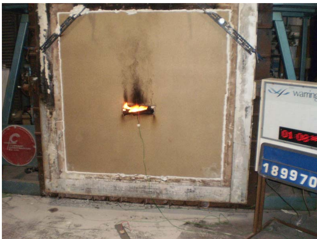
The unexposed face of the assembly after a test duration of 68 minutes
