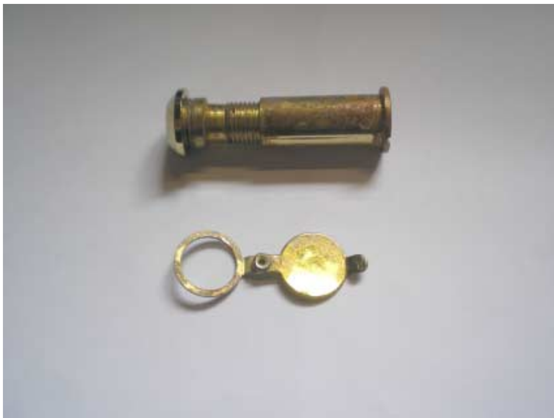
CILPVD – Post Corrosion Grade 4
