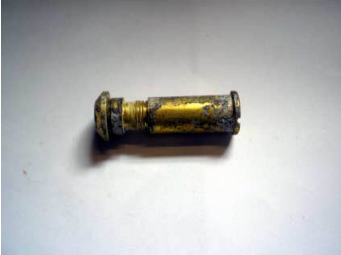
CILGA – Post Corrosion Grade 4
