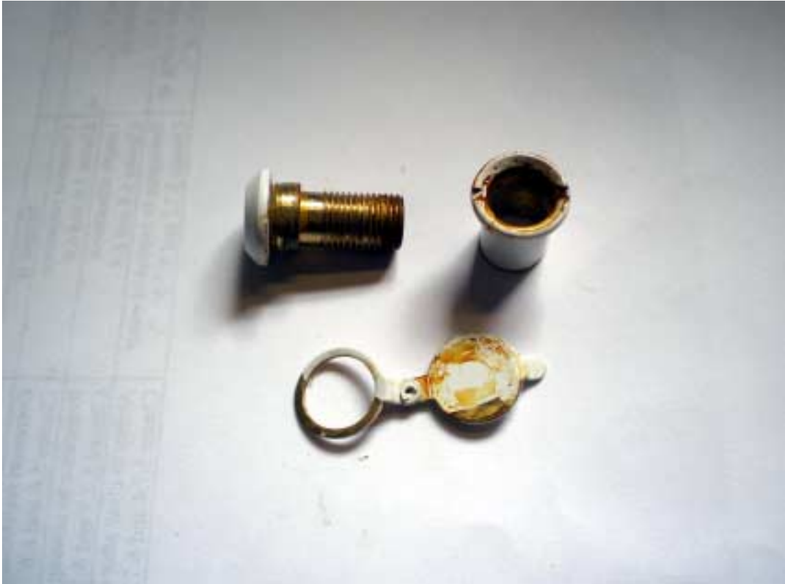
CICWH – Post Corrosion Grade 4
