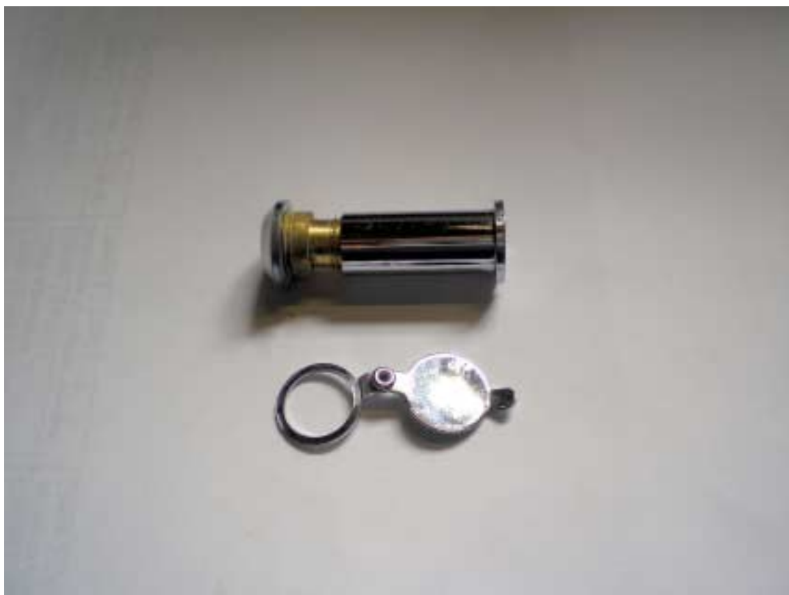
CILCH – Post Corrosion Grade 4
