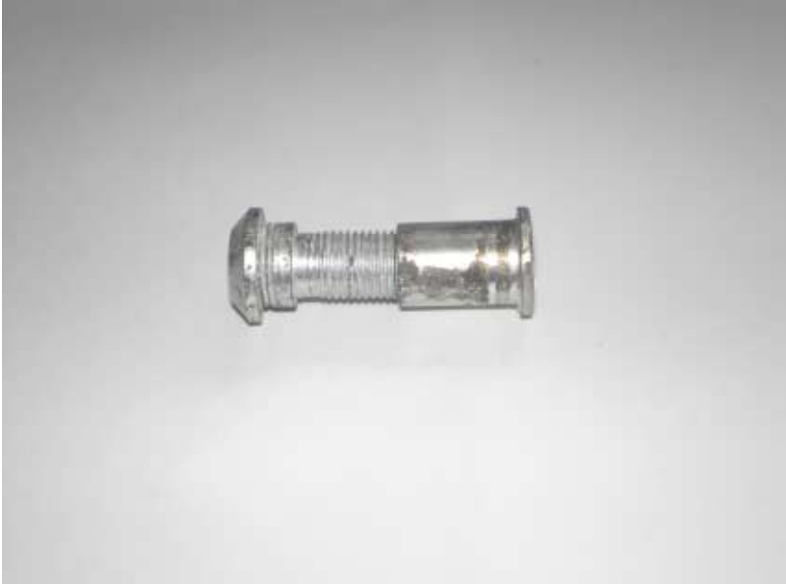
CILSA – Post Corrosion Grade 4
