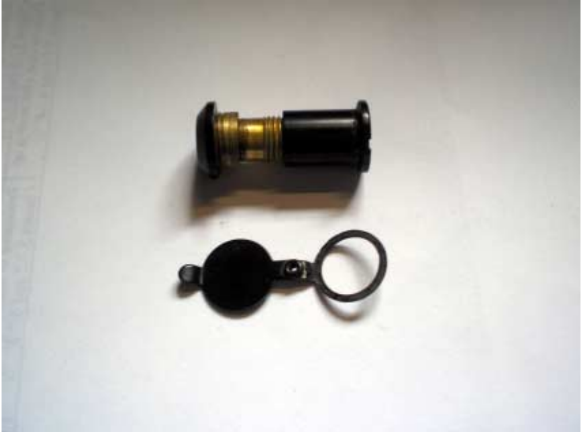
CICBL – Post Corrosion Grade 4
