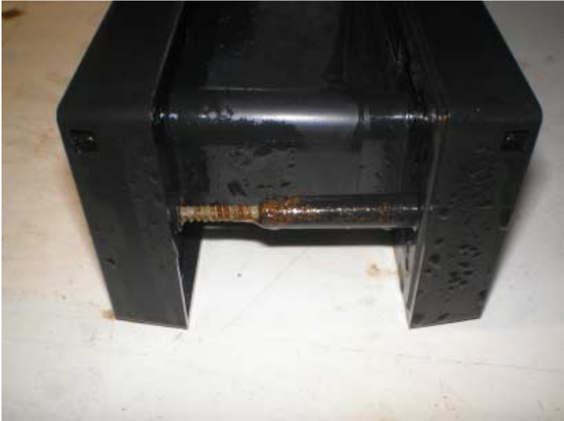
Corrosion of Type A Fixing
